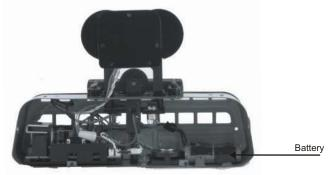
To gain access to replace the battery please follow the body side remove instructions under the car light bulb replacement instruction section on page 19.
