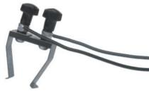
6) Install Lock-on by squeezing Lock-on fingers, inserting them between the rails and release. Connect wires to transformer with top rail wire to ground(-) and the bottom rail wire to positive (+). This wiring configuration is important for proper operation of the contemporary models when operating with the MTH DCS System.
