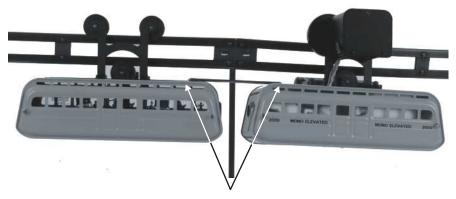
To couple or connect the cars together insert ends of the drawbar into the drawbar holes on the roof of each car
