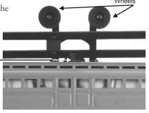
3) Release tension from contact roller and latch contact roller lock.
