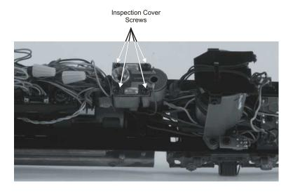
Figure 17. Inspecting the Smoke Unit Wick
