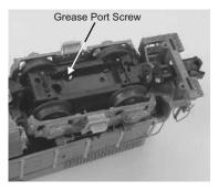
It is recommended to lubricate the outside truck block idler and drive gears with grease. Use the diagram shown in Figure 11 below as a guide and add grease to the points marked.
