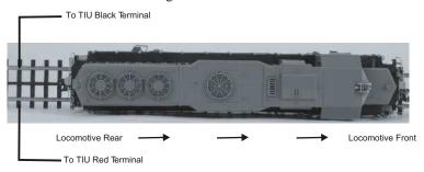
Figure 5: Proper 2-Rail polarity wiring and locomotive orientation
