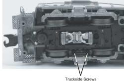
Figure 12. Truckside Screws
