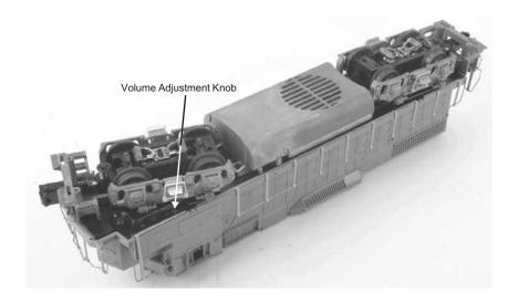
Figure 7. Manual Volume Adjustment Knob
