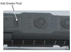
Figure 16. Filling The Smoke Unit
