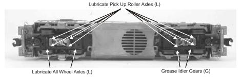
Figure 8. Lubrication points on the Locomotive
