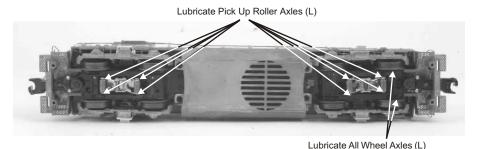
Figure 1. Lubrication Points on the Locomotive
