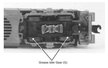
Figure 11. Greasing The Idler Gears
