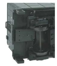
Figure 5: Pre-drilled Kadee® Coupler mounting holes
