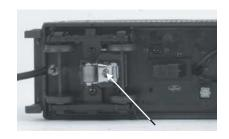
Figure 1: 3-Rail Pickups installed with a single Phillips Screw
