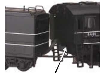
Plug Tender Plug into Dollar Socket at back of cab. Figure 1a. Connect the Tender to the Engine
