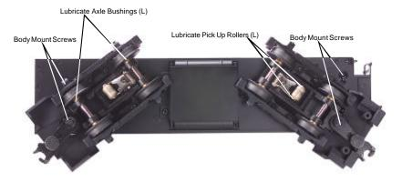
Figure 1: Lubricating The Chassis
