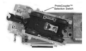
Figure 5: Proto-Coupler Selection Switch
