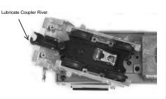
Figure 3: Lubricating The ProtoCouplers
