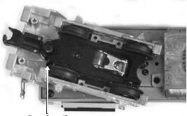
Proto-Sound® Volume Control Figure 4: Adjusting The ProtoSound Volume and selecting the ProtoCoupler<sup>™</sup>
