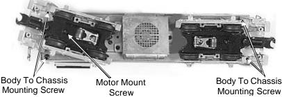
Figure 7: Lubricate The Tender Chassis Trucks
