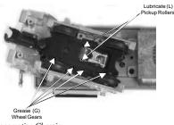
Figure 6: Lubricating The Locomotive Chassis
