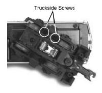
Figure 11. Screws to Remove to Access the Traction Tires
