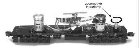
Figure 12. Location of the headlamp in the Engine.
