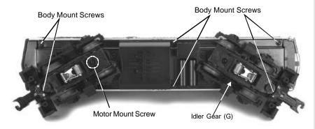
Figure 10. Body Mount Screws and Greasing Points.
