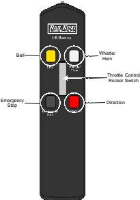
Fig. 6: Overview of the Remote controls
