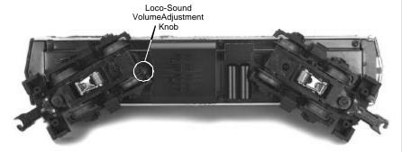
Figure 8. Location of the Loco-Sound Volume Adjustment Knob
