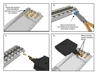
Fig. 1a-1d: Installation of Remote Lock On
