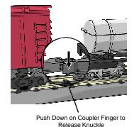
Figure 4. Coupling the Freight Cars Together
