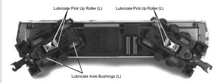
Figure 9. Lubrication Points on the Engine
