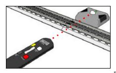
Figure 5. Aim the Remote at the Rounded Side of the Receiver's Lens, the Slanted Side Should Face Away.
