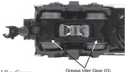
Greasing The Idler Gears
