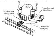
Figure 8: Wiring Up A Bell Button Controller
