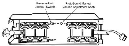
Figure 6: Adjusting The ProtoSound Volume
