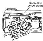
Figure 2: Smoke Unit On/Off Switch
