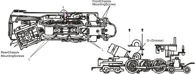
Figure 8: Lubricating The Locomotive Chassis
