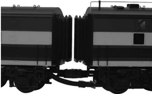
Figure 5: Correct way to Connect wire harness plug into the receptacle [The top of the plug will have the word 'TOP' imprinted on it]
