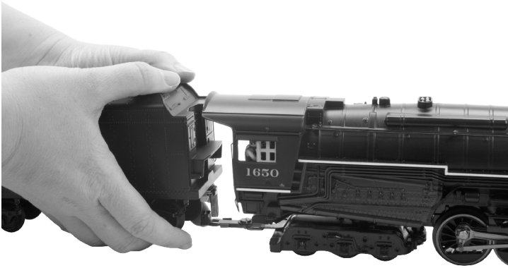
Figure 4: Connecting Locomotive to Tender
