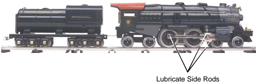
Figure 2: Lubricating Side Rods
