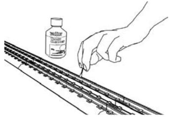
To clean the track, use RailKing Track Cleaning Fluid found in Maintenance Kit (30-50010) or denatured (not rubbing) alcohol and a clean rag. Unplug the transformer and wipe the rails of the track, turning the rag frequently to ensure that you are using clean cloth on the rails. Thereafter, keep an eye on the track and clean it when it gets dirty to ensure good electrical contact and to lengthen the life of the tires.
