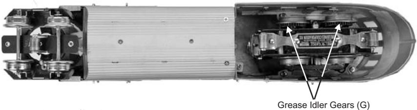
*Figure 8: Grease Idler Gears*
