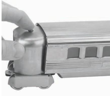
*Figure 4: Step 4 [Locking Vestibule in Place]*
