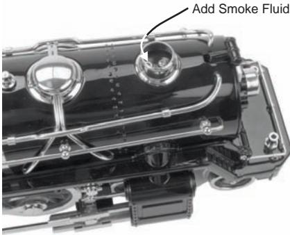
If you choose not to add the fluid (or have already added the fluid but choose to run smoke-free), turn off the smoke unit off by turning the smoke volume control to the minimum setting (counterclockwise). The smoke volume control is located underneath the engine (see below). **Failure either to add fluid to the unit or to turn it off may damage the smoke unit heating element and/or wicking material.**
