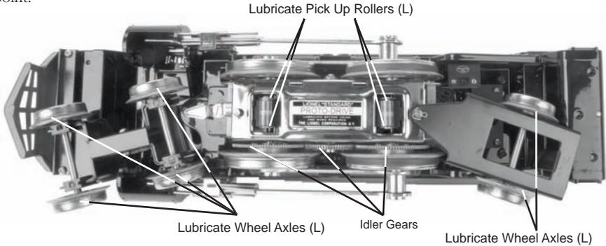
The locomotive's internal gearing was greased at the factory. Grease engine every 50 hours of use or at least once yearly if engine is not run. Use a lithium based grease and follow the greasing instructions.
