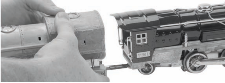
Fig. 4: Pushing Connectors Together
