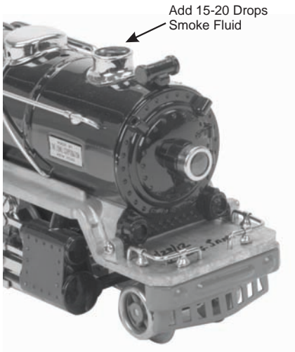
Fig. 2: Adding Smoke Fluid
