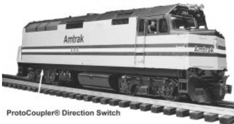
The 3-rail models are controlled by two DCRU™ electronic reverse units. The reverse unit operates in the same manner that all reverse units function by using forward, neutral and reverse states that are entered each time the throttle is turned on and off or by using the transformer direction switch (if so equipped). The 2-rail model's direction is controlled through the polarity of the DC power source and operate the same as all 2-rail DC engines.
