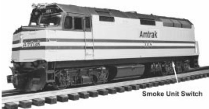
Figure 2: Smoke Unit Switch Location
