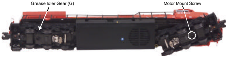
Figure 7. Locations of Greasing Points on the Locomotive
