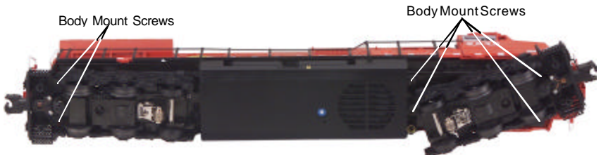
Figure 6. Locations of the Body Mounting Screws
