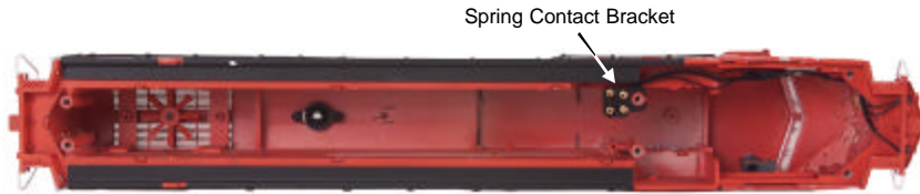
Figure 10. Replacing the Lights Mounted on the inside of the Shell
