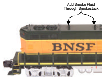
Figure 2. Add Smoke through the Smokestack
