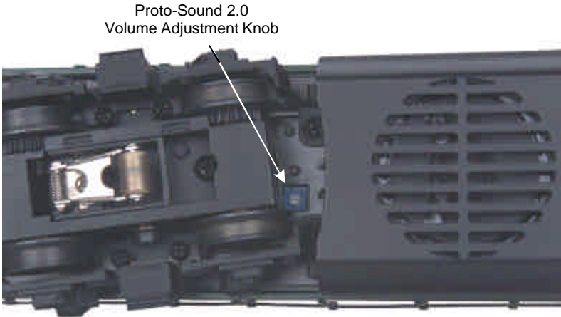
Figure 4: Manual Volume Adjustment Knob
