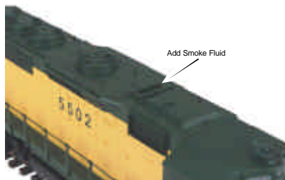
Figure 10: Adding Smoke Fluid
