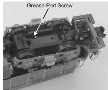
It is recommended to lubricate the outside truck block idler and drive gears with grease. Use the diagram shown in Figure 11 below as a guide and add grease to the points marked.
