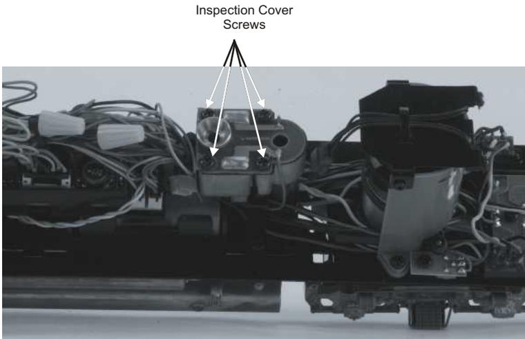
*Figure 17. Inspecting the Smoke Unit Wick*
