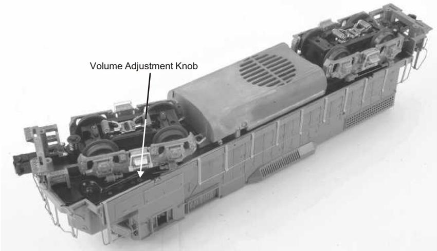
*Figure 7. Manual Volume Adjustment Knob*
