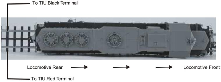
Figure 5: Proper 2-Rail polarity wiring and locomotive orientation
