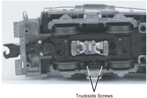
*Figure 12. Truckside Screws*
