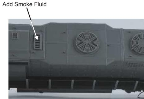
*Figure 16. Filling The Smoke Unit*
