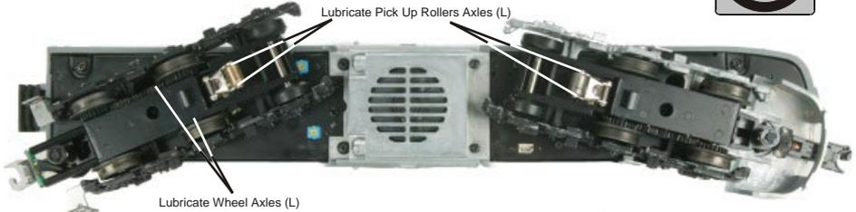
*Figure 5. Lubrication Points on the Locomotive.*
