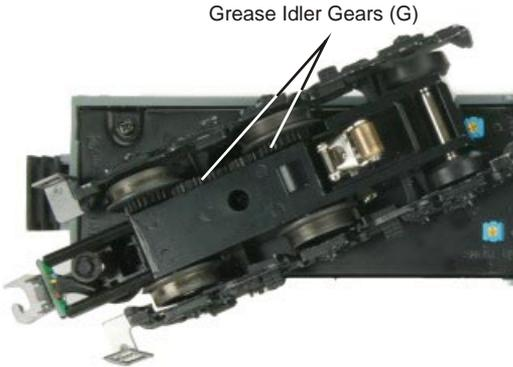
*Figure 7. Greasing The Idler Gears*
