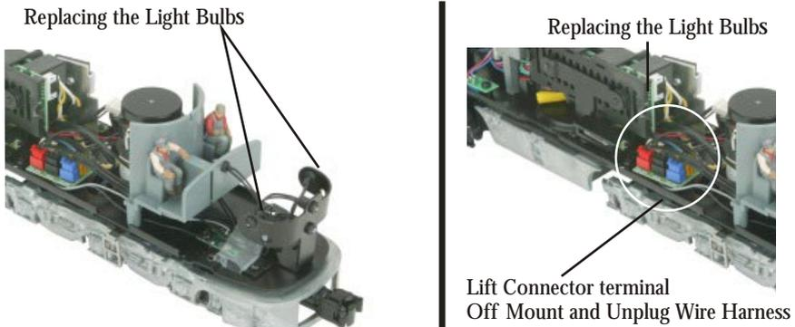
*Figure 8. Replacing the Light Bulbs*
