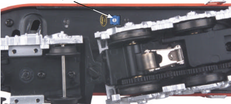
Figure 2: Proto-Sound Manual Volume Adjustment
