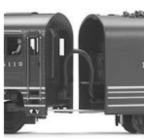
Figure 1: Plugging in the tender harness
