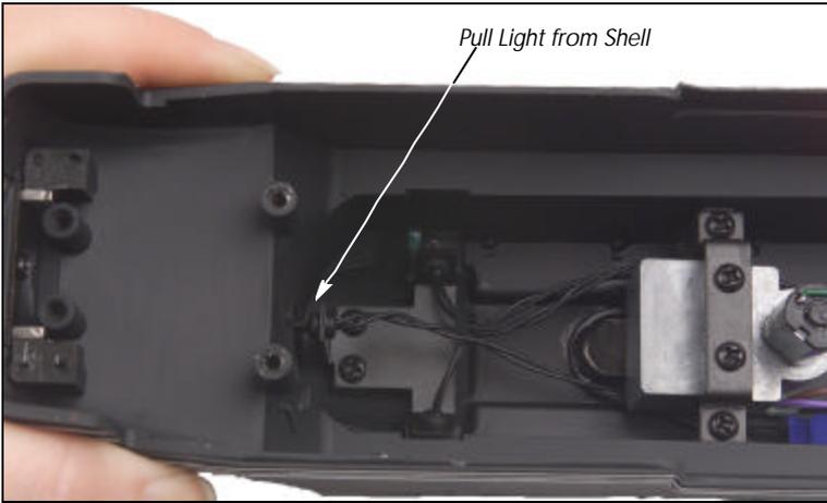
Figure 7 - Replacing the Headlight
