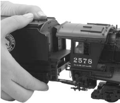
Figure 5: Connecting Locomotive to Tender
