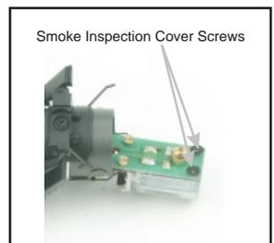
Figure 9: Smoke Unit Inspection Cover
