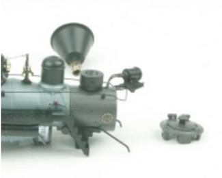
Figure 10: Replacing the Headlight
