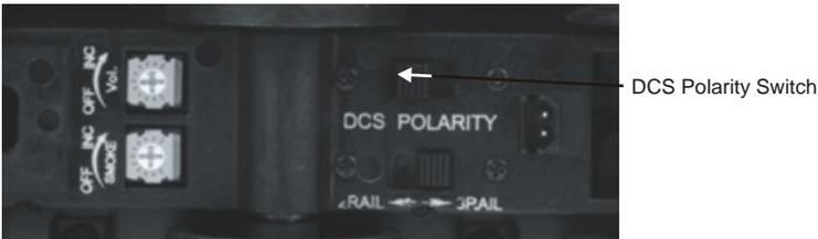
*Changing the polarity with the locomotive polarity switch*
