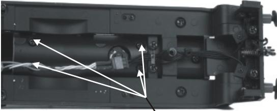
Remove Screws to access smoke unit
