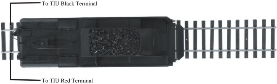
*Proper 2-Rail polarity wiring and locomotive orientation (Reference photo)*
