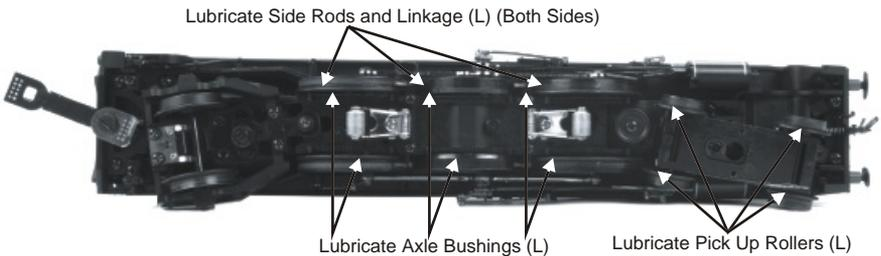
*Lubrication Points on the Locomotive*
