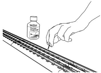
To clean the track, use RailKing Track Cleaning Fluid found in Maintenance Kit (30-50010) or denatured (not rubbing) alcohol and a clean rag.
