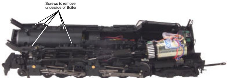
Figure 8. Screws to remove the top of the boiler..
