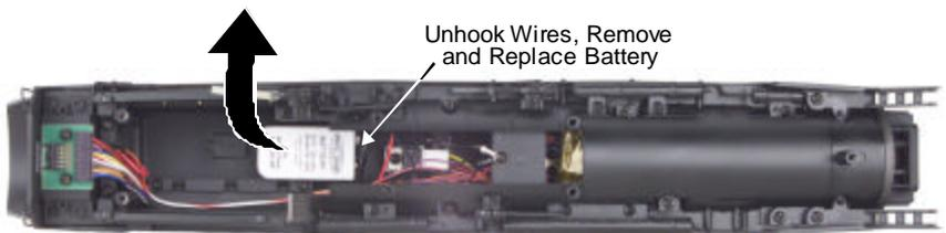
*Figure 11. Replacing the Battery*
