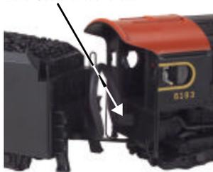
Figure 1a. Connect the Tender to the Engine
