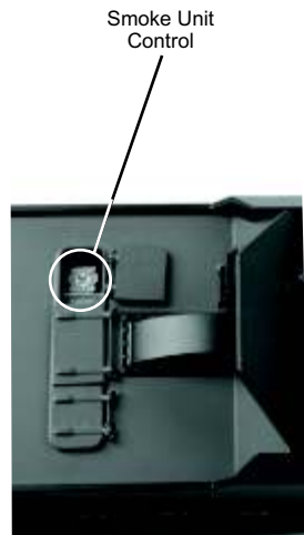
Figure 2: Smoke Unit Control Location
