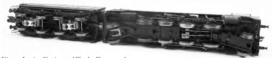
Figure: Laying Engine and Tender Down to Access
