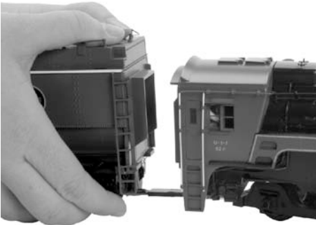
Figure 5: Connecting Locomotive to Tender
