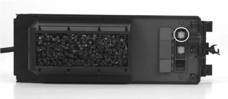
Figure 2. Manually Adjusting the Proto-Sound 2.0 Volume
