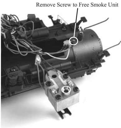
Figure 5a. Accessing the Smoke Unit
