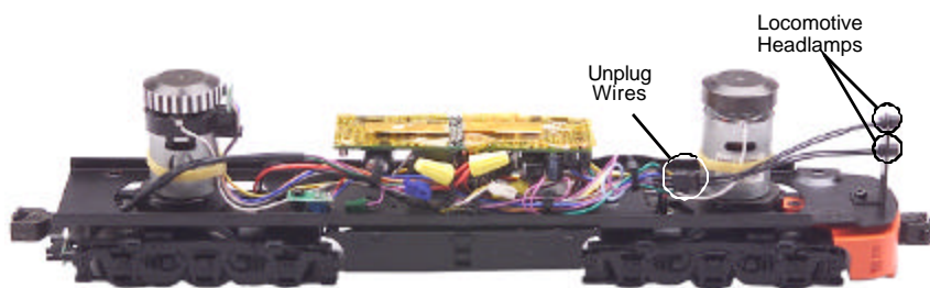
Figure 5. Location of the headlamp in the Engine.
