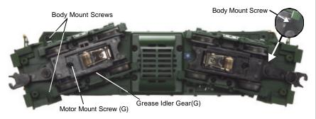
Figure 3. Lubrication Points on the Engine
