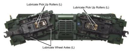
Figure 2. Lubrication Points on the Engine
