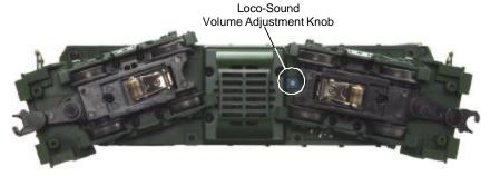
Figure 1. Location of the Loco-Sound Volume Adjustment Knob
