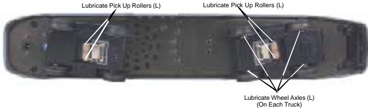
Figure 1. Lubrication Points on the Locomotive
