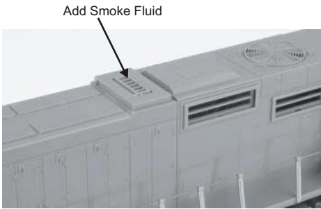
Figure 7. Filling The Smoke Unit
