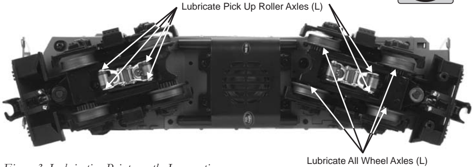
Figure 3: Lubrication Points on the Locomotive
