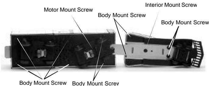
Figure 5: Removing The Body From The Chassis
