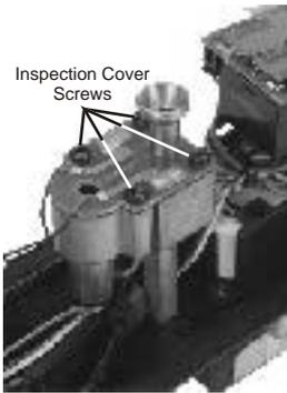
*Figure 9. Inspecting the Smoke Unit Wick*
