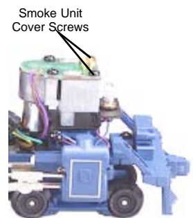
Figure 6. Smoke Unit Inspection Cover
