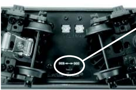
Figure 6: Changing from DCS to DCC Mode
