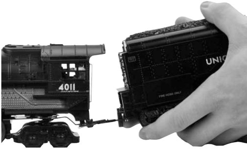
Figure 4: Connecting Locomotive to Tender
