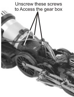
Figure 7. Motor Gearing Grease Plate Screws
