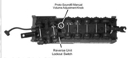
Figure 6: Adjusting The ProtoSound® Volume
