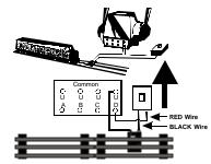
Figure 7: Wiring Up A Bell Button
