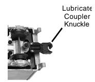
Figure 5: Lubricating The Coupler
