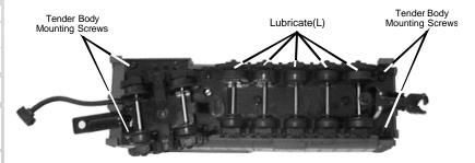
Figure 9: Lubricate The Tender Chassis Trucks
