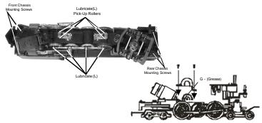
Figure 8: Lubricating The Locomotive Chassis
