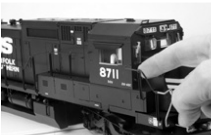
Figure 18: Handrail Separation From Cab
