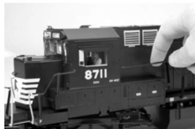
Figure 19: Handrail Separation From Cab
