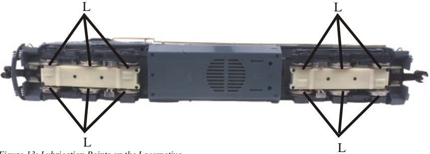
Figure 13: Lubrication Points on the Locomotive
