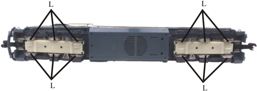
Figure 6. Lubrication Points on the Locomotive
