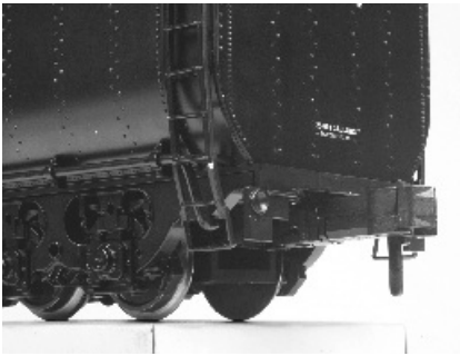
Figure 1a: MTH ProtoCoupler in higher position.
