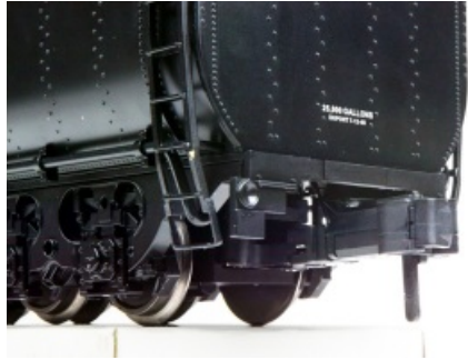
Figure 1b: M.T.H. ProtoCoupler in Lower Position.
