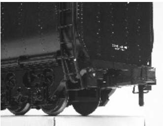
Figure 3: Shorten locking pin when coupler is in lower position.
