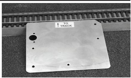
***Note:** The metal template should be placed against the rails closest to the mast location. The rails were chosen as reference to avoid variances since some layouts have track with built in roadbed or those that may have ballast applied as opposed to track without roadbed or ballast.*
