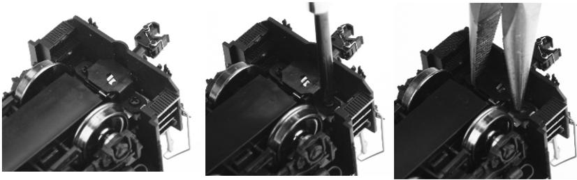
Identify & Remove Mounting Screws
