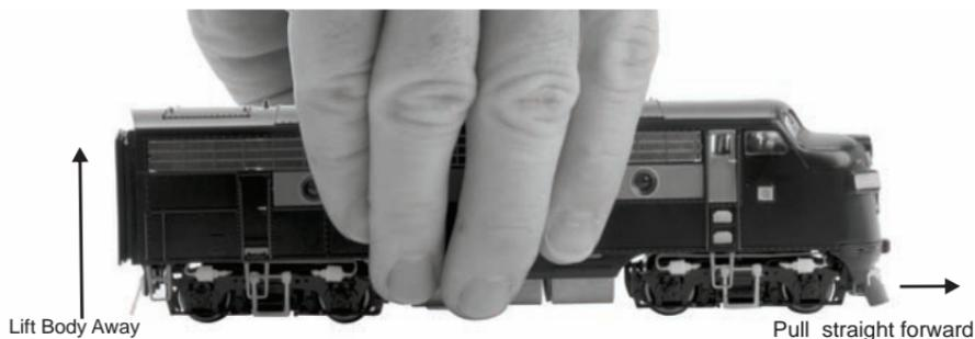
You may find it easier or necessary to remove the pilot before removing the body. To remove the pilot, carefully pry out each end of pilot to release the snaps then pull pilot straight forward from the body. Be careful not to bend or break the steps.
