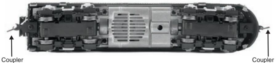
1. To remove the couplers, use a phillips head screwdriver to remove the screws.
