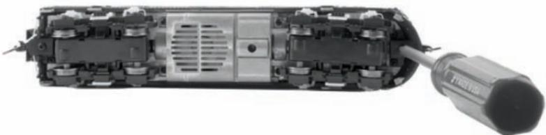
2. Once the screws are removed, you can pull away the coupler, for the A Unit you will have to pull the coupler through the pilot.
