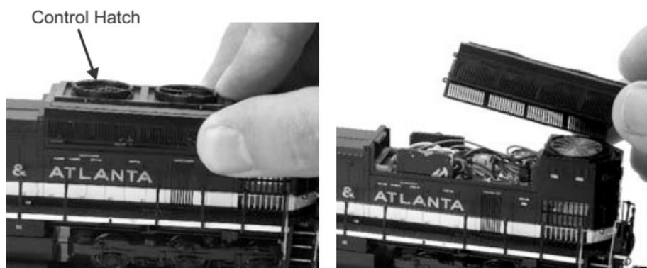
To remove the Control Hatch, gently pull it outward and lift it off from the side.
